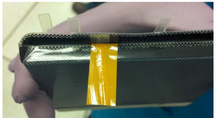
Figure 22: Edge Fold on Vent Side
