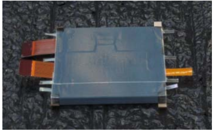
Figure 20: First Fold of Tamper responsive sensor on Inner Cover
