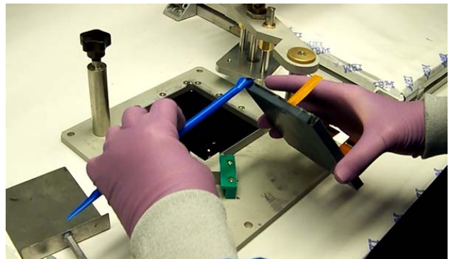
Figure 25: Applying Resin to Package Corners
