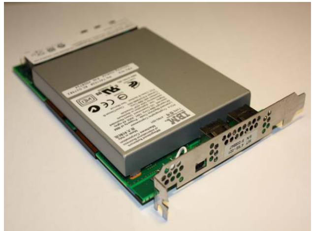
Figure 29: Finished Cryptographic Module assembled to PCIe Card
