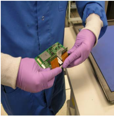
Figure 6: Flex Cable Pre-Bending
